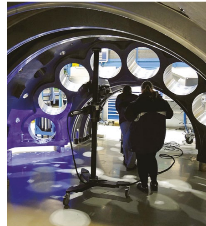
Measurement of the real geometry of a turbine housing using laser scanning
